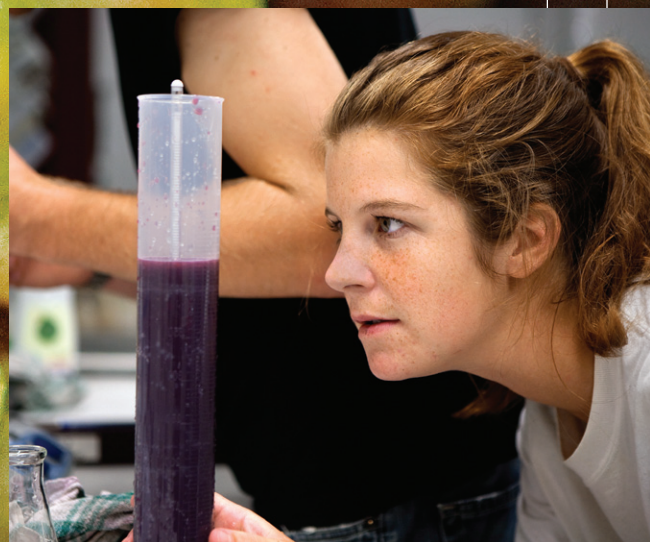
Macy Stubstad '12 uses hydrometry to measure soluble solids present in a cabernet franc.
