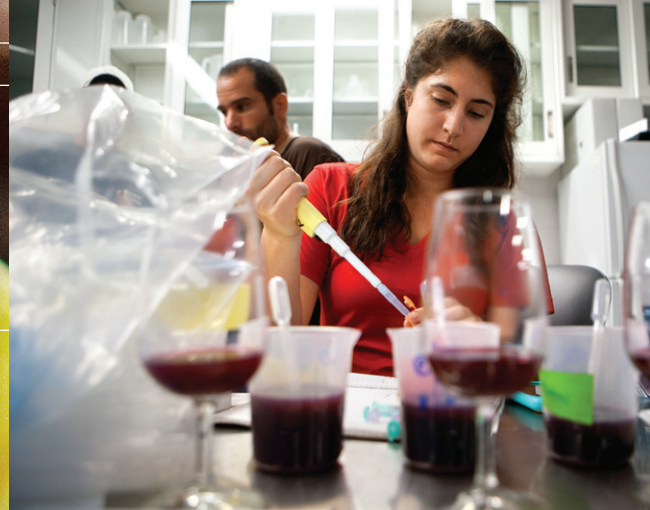
Amanda Vondras '11 dilutes samples of her wines in cuvettes to measure wine color (amount of pigment). The samples will be analyzed by a spectrophotometer.
