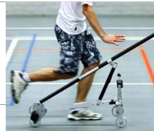
An experimental bicycle designed to eliminate the gyroscopic effect of spinning wheels and the "trail" of the front wheel is still stable on its own, disproving conventional theory.
